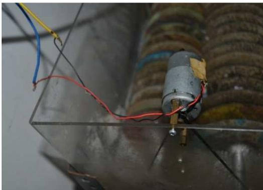
Gambar 1 Reaktor Rotating Biological Contactor
